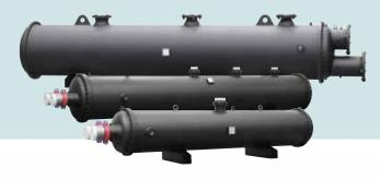
With a flooded evaporator, a pool of refrigerant is maintained in the shell, submerging the tubes to a set level. As the refrigeration load varies, a refrigerant-level control acts to maintain the liquid level in the shell. The refrigerant pool in the shell behaves as a flywheel, allowing the controls of the flooded evaporator to successfully track the varying load of a batch process.
