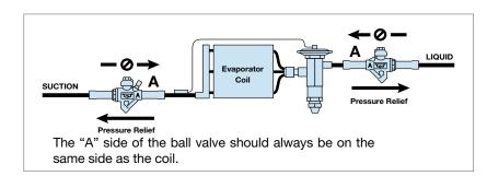
The EBV(T)-PR valve will close in one direction and relieve pressure in the other direction. This single valve would replace a current ball valve plus a check valve plumbed around the ball valve. Allows evaporator coil to be isolated without over pressurizing due to warm up. May also have needs in loop piping and at the rack.
